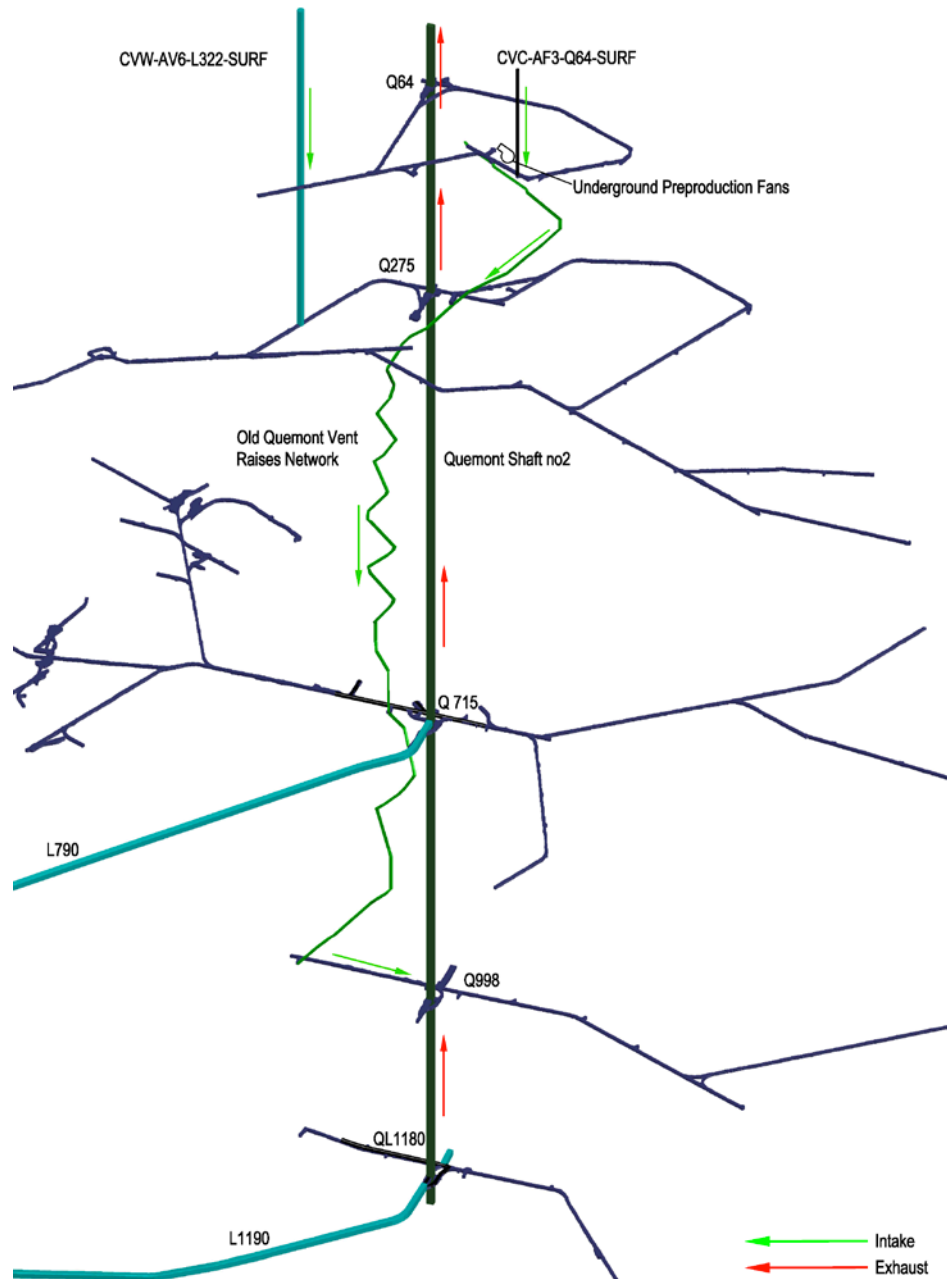
Figure 16-35: Complete preproduction/development ventilation network
