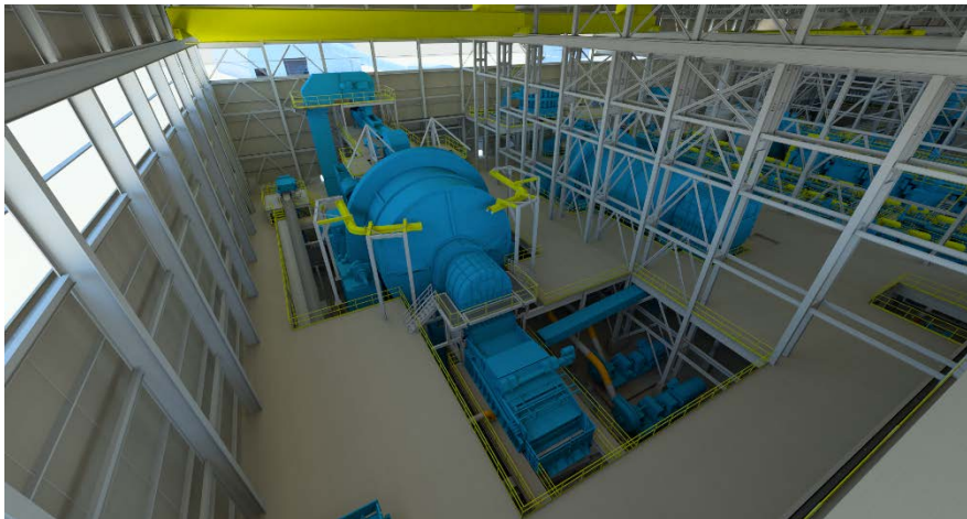
Figure 17-5: 3D model arrangement of the SAG mill and ball mill circuit
