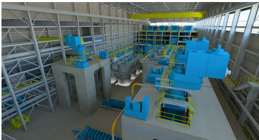
Figure 17-10: Configuration of the pyrite concentrate regrinding circuit
