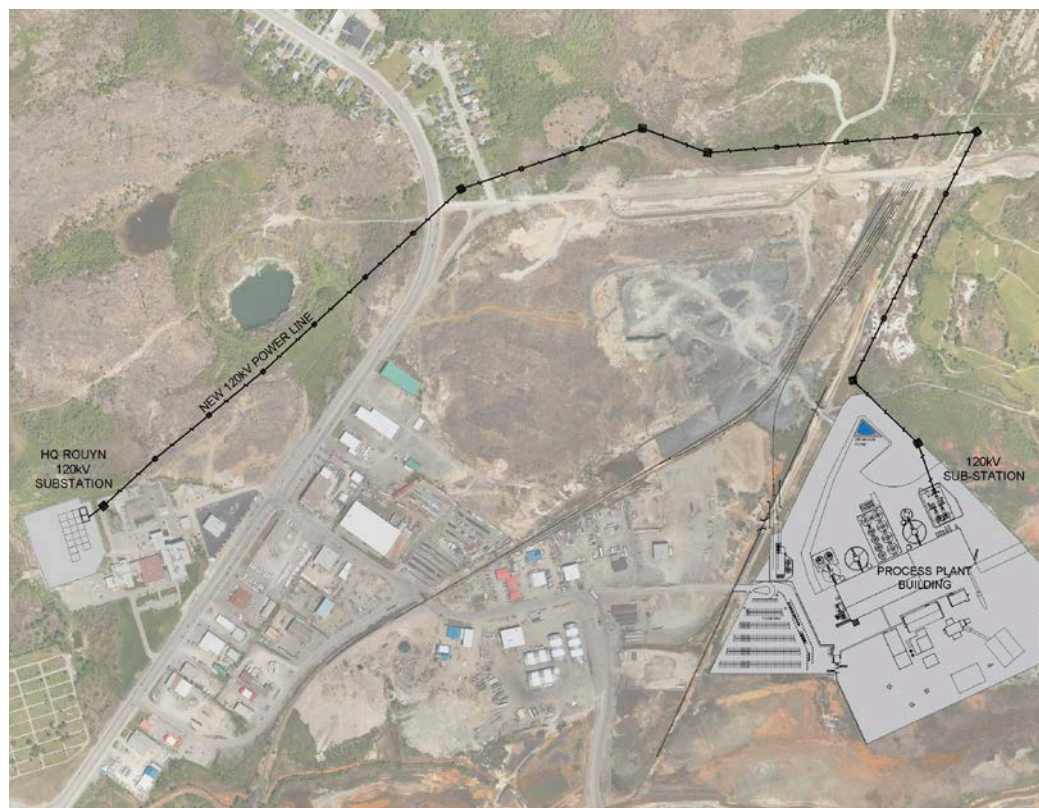
Figure 18-5: Proposed overhead line from the Hydro-Québec Rouyn-Noranda substation to the Mining Complex
