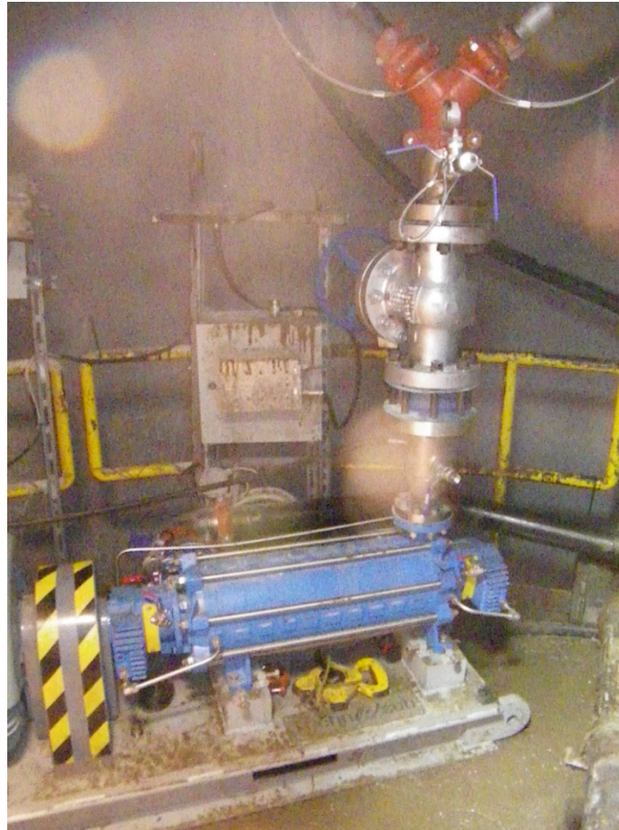
Figure 16-13: Typical booster pump installed on a Galloway
