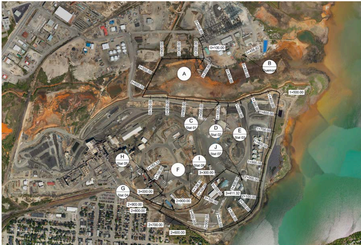
Figure 16-70: Proposed surface slurry pipeline on Horne property
