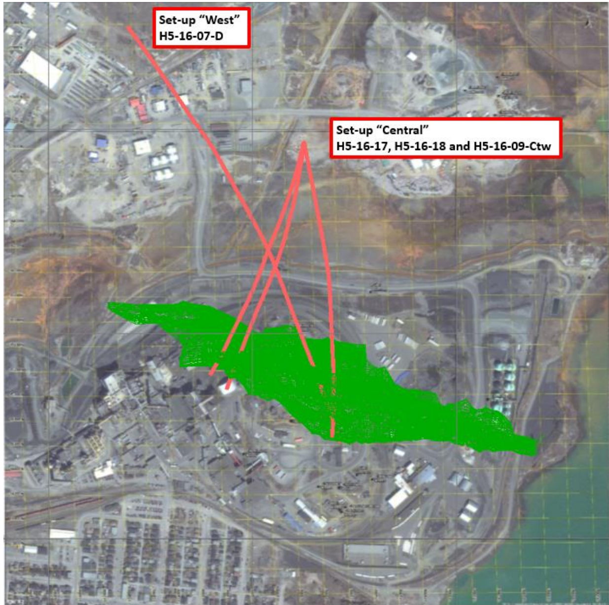
Figure 10-1: Location map of the confirmation drill holes realized in 2016 showing the projection of the main mineralized envelope (ENV_A)
