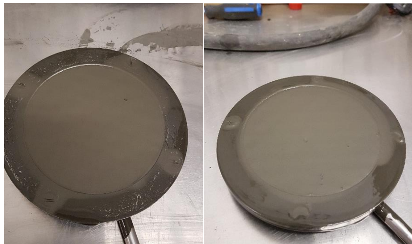
Figure 13-57: 50/50 PFT/PCT vacuum filtration cakes – 53.5% w/w slurry feed (left) and 60% w/w (right)
