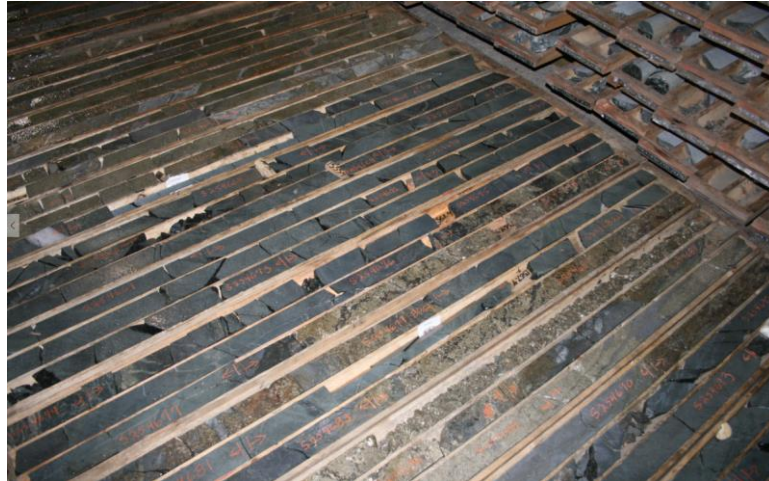
Figure 12-3: Half-core witness samples from mineralized zones
