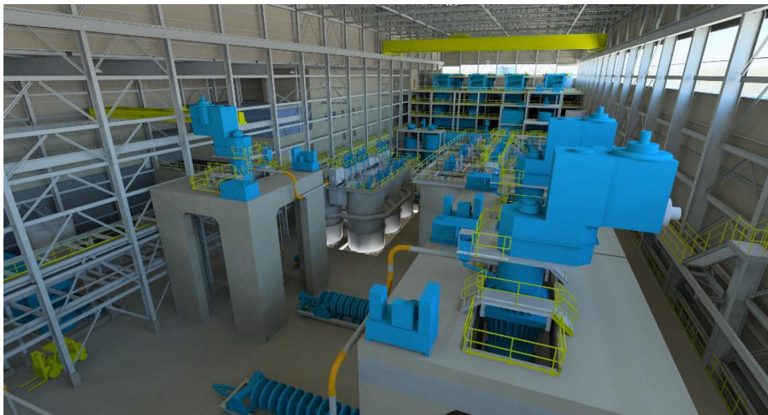
Figure 17-9: Configuration of the pyrite concentrate regrinding circuit
