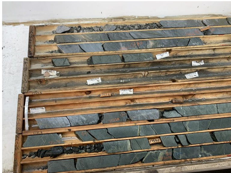
Figure 12-4: Half-core witness samples from mineralized zones with interval missing for metallurgical testing purpose
