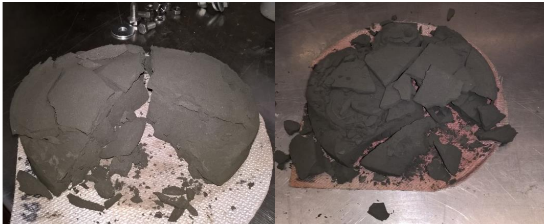
Figure 13-58: Filtered cake of 100% PFT and 50/50 PCT/PFT
