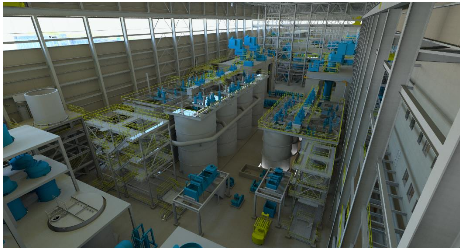
Figure 17-11: Configuration of the CIP and gold recovery circuits
